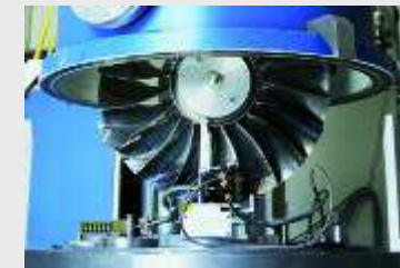
Local heat treatment by induction
